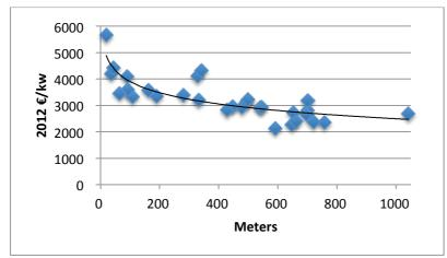
Figure 3: Relation between net head and CAPEX in our data sample.
